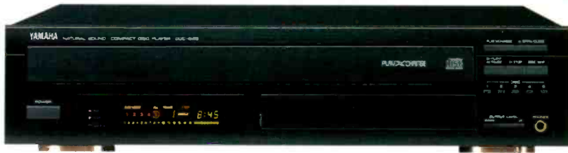
Yamaha's CDC-845 five-disc carousel ($499) shortens track-switching time in random-play and programmed-play modes by memorizing a disc's contents on the first pass.
