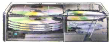
Since the CD only partially extracts during playback, response is faster and less space is required.
