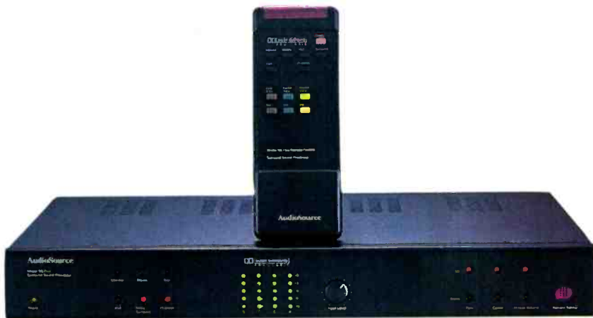
AudioSource's SS Five add-on surround-sound processor ($350) uses a highly regarded Dolby Pro Logic decoding chip from Analog Devices. It has a subwoofer line output and three 24-watt amplifiers for driving the center and surround speakers.
