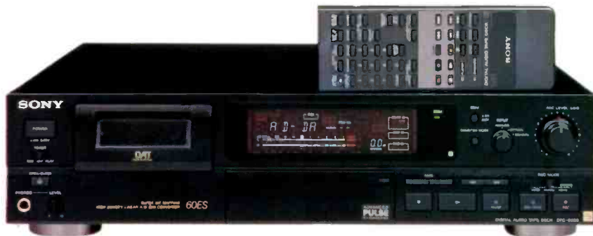
The Sony DTC-60ES DAT deck ($1,200) uses 1-bit A/D and D/A converters and has both optical and coaxial digital inputs and outputs. It also includes the company's Super Bit Mapping (SBM) system, which can reduce perceived noise in recordings made through the analog inputs by shaping the noise spectrum according to the ear's varying sensitivity across the frequency band.
