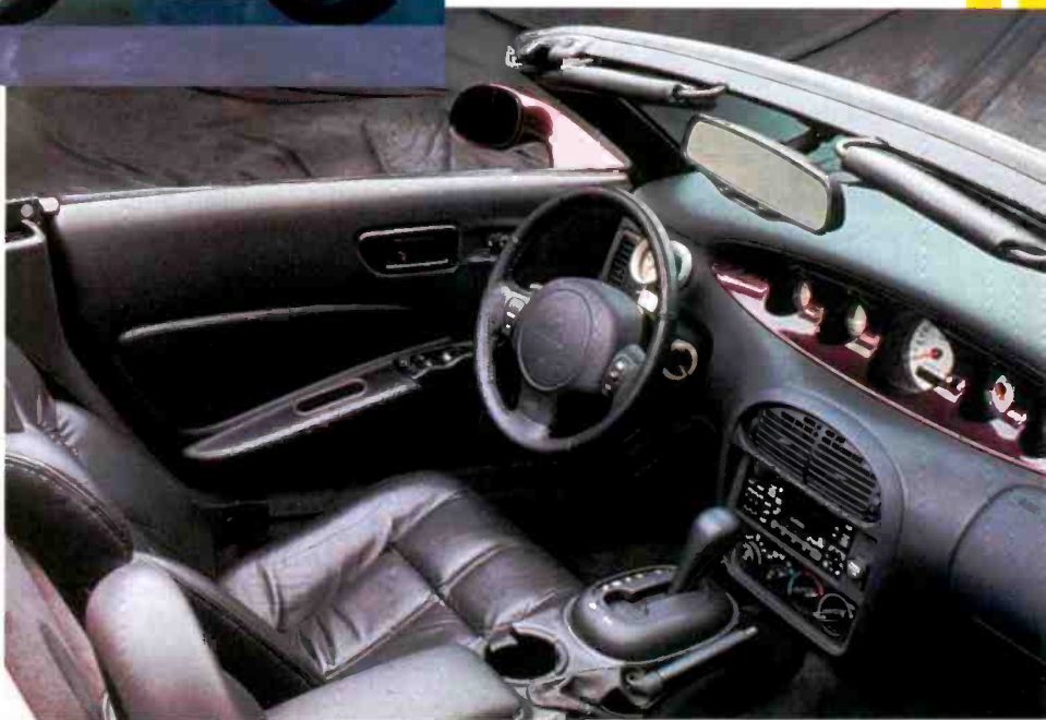
Plymouth's new retro-style Prowler roadster comes with a seven-speaker Infinity sound system that features fixed EQ for top-down driving, steering-wheel audio controls, and a cassette head unit that controls a six-disc CD changer.
