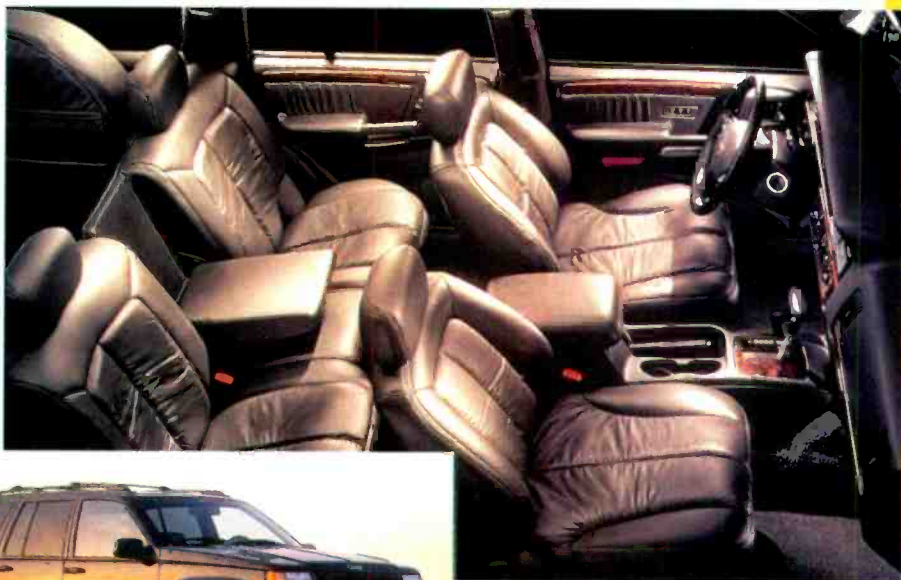
Standard in the Jeep Grand Cherokee 5.9 Limited is an Infinity Gold System comprising a CD/cassette head unit, a 180-watt amplifier, custom equalization, ten drivers, and steering-wheel audio controls.
