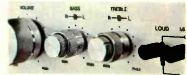
Clutched bass and treble controls with detents.
