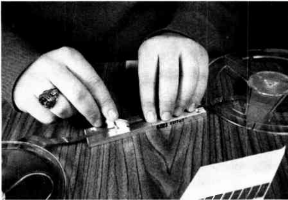
Edittall splicing-block channels hold tape while mitre groove guides razor blade for precise cut.
