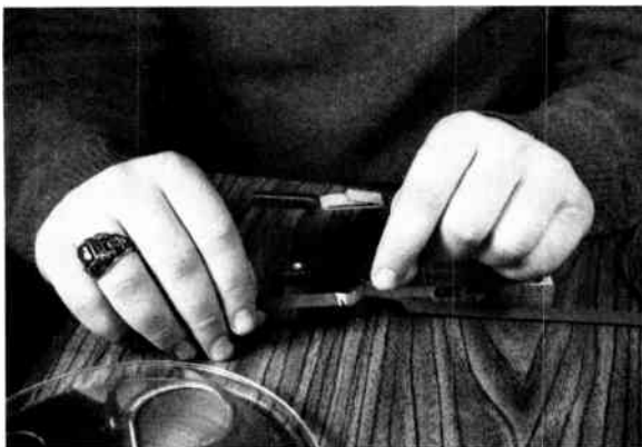
With tape removed from block, backing is peeled from splicing tape, thus completing the splice.
