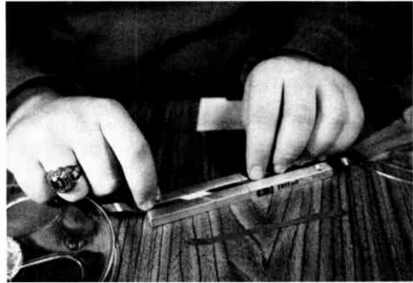
After ends of tapes are butted on diagonal cuts, pre-cut splicing tape is centered and pressed on.
