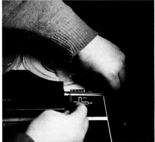
Precisely measured distance from playback head gap is used for marking tape for cutting.
