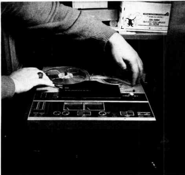
With cue or pause control engaged, reels can be hand-turned to locate nulls for cutting tape.
