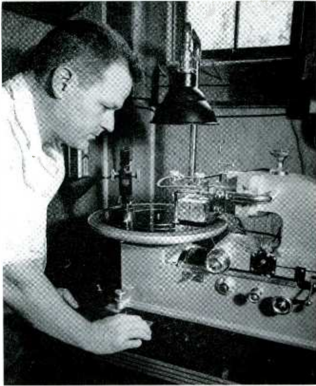
Emory Cook cuts a binaural disk on a Special Scully lathe.
