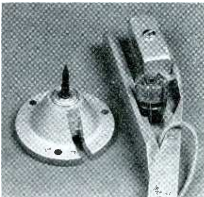
Fig. 2. Base and arm spring mechanism.
