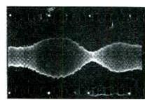
Fig. 7. Sound level, at three low frequencies, as microphone was moved across room in Direction C, Fig. 4. Distance of travel: about 10 ft.
