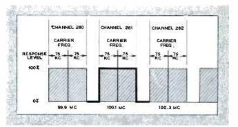
Fig. 2. The frequency response characteristics of the ideal tuner wound exactly match those of the broadcast station, shown in Fig. 1 and indicated above by the heavy line.
