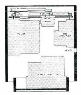
Fig. 2. These two drawings show exact placement and overlapping of components. The left hand view is a cross-section as seen from front.
