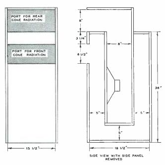
Fig. 5. Folded Air Coupler designed by O. C. Hoggren.
