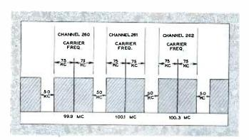
Fig. 1. Channels used by FM broadcast stations are centered around a carrier frequency with a 75 kilocycle band on either side of the carrier. A 50-kc. band separates channels.
