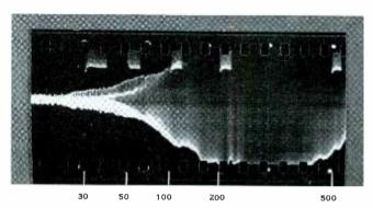
Fig. 10. Speaker mounted in window, facing outside for free-field conditions. There are traces of frequency doubling and trebling up to 75 cycles. The bass resonance is almost damped out by the high flux density of the magnet—13,000 lines.
