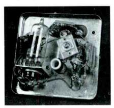
View of underside of oscillator Fig. 3. View of underside of oscillator chassis. Tube at left is 6AT6. Almost in center is oscillator coil, which is slug tuned. Trimmer capacitor is just above coil.
