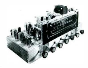
Browning model RJ-20A FM-AM tuner. Controls: on-off; tuning, separate bass and treble tone controls; volume; AM frequency bandwidth; selector switch providing AM, FM, and three spare positions. Armstrong circuit. AFC.
