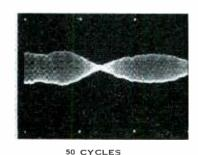
Fig. 6. Sound level as microphone traveled diagonally, Direction B.
