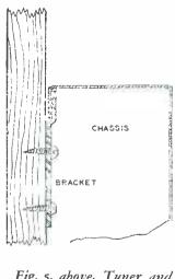
Fig. 5, above. Tuner and preamplifier chassis are booked over brackets.
