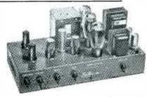
Kits supplied with punched chassis, finished in bronze hammertone, with control designations silk screened on the front panel; all necessary components; transformers and choke; tubes. Easy to follow instruction book containing stepby-step instructions, schematic and pictorial diagrams.
