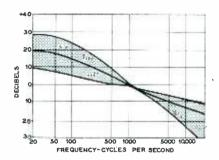
Fig. 5. Control range for AES PHONO input.
