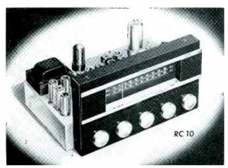
Radio Craftsmen model RC-1). Comtrols: separate bass and treble tone controls; on-off and volume; tuning; input selector which provides three spares. Built-in phono preamplifier for magnetic cartridges. Armstrong circuit. AFC.
