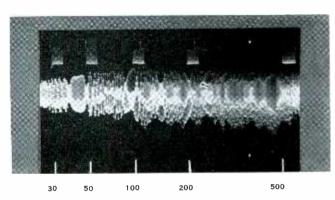
Fig. 13. Same as Fig. 11, but cabinet placed in centre of room. Room effects swamp the picture here. Probably a fairly true representation of what we normally hear.
