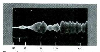
Fig. 11. Speaker mounted in matched reflex cabinet, placed in corner of room. The corner position helps to produce a rise in reflex output below 50 cycles. The severe dips at about 130 and 260 cycles are probably phase cancellation effects. Note start of room reflections at 220 cycles.
