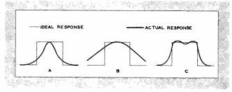
Fig. 3. In actual practice, tuning characteristics shown in A, B, C, above, are achieved. Both A and B are poor; C balances wide frequency response against good sensitivity.
