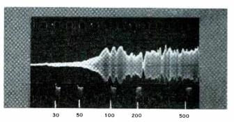
Fig. 12. Same as Fig. 11, but cabinet placed 4 ft. from corner. The more central position shows room reflections at about 100 cycles. The 40-cycle hump of Fig. 11 has disappeared.
