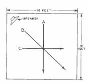
Plan of test room, with direction of microphone travel.
