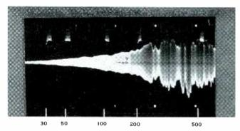
Fig. 9. Speakers mounted on 2 ft. baffle, placed in centre of room. Note the severe loss of bass which starts around 200 cycles as a result of small baffle area, incidentally cancelling cone resonance and removing frequency doubling. Suitable mounting for clean reproduction of speech.
