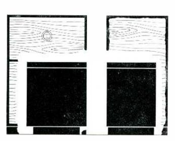
motor board is mounted on soft rubber.
