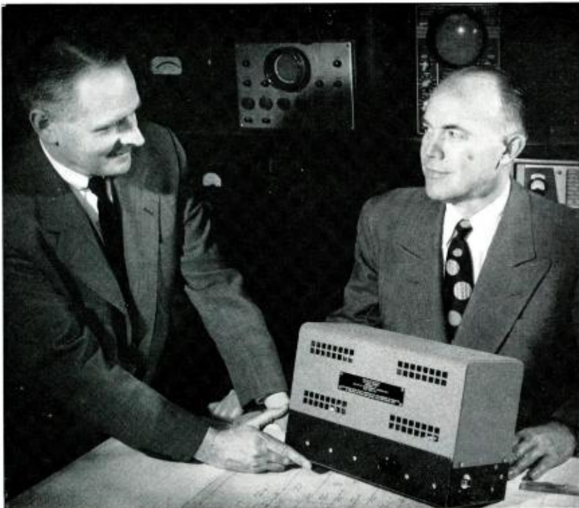
The Stereosonic system makes it possible to transmit two separate audio channels from one FM station. At the receiving end, an ordinary FM set and a Stereosonic multiplex adapter, illustrated here, provides the separate outputs for two separate amplifiers and speakers. William S. Halstead, left, and Murray G. Crosby are responsible for the development of this system, first demonstrated to the Federal Communications Commission in 1950 over station W'GNY.
