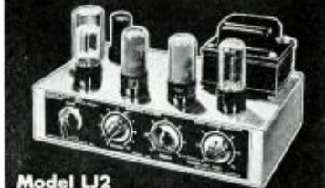
Model LJ2 Power output, 8 watts, 18 watts peak. Distortion at 8 watts, 1.1% harmonic and 4% intermodulation. Frequency response: 5, 100, 20 to 20,000 CPS, at 3 watt level. $36.50
