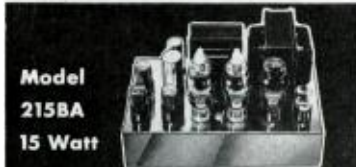
Model 215BA 15 Watt ALL TRIODE BASIC AMPLIFIER Response 10 to 100,000 CPS. Peak power 24 watts. Distortion at 8 watts, .07% H. and .2% I.M. 25 DB feed-back from 3 loops, 2 direct coupled stages, cathode follower drivers. $99.50
