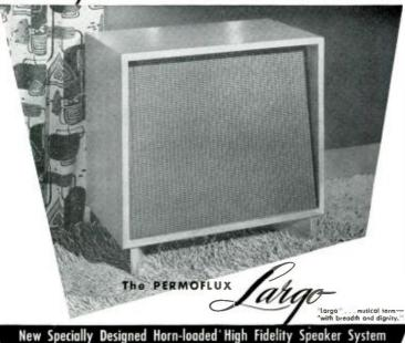
The Largo is a complete wide range speaker system utilizing the new Permoflux 8V81 Super Royal Eight speaker and 32 KTR Super Tweeter in an acoustically advanced enclosure scientifically matched to the speaker characteristics. The enclosure is an entirely new and unique horn-loaded non resonant baffle with horn loading of the speaker back wave accomplished in the cabinet base. Every inch of the cabinet construction serves an acoustically useful purpose.
