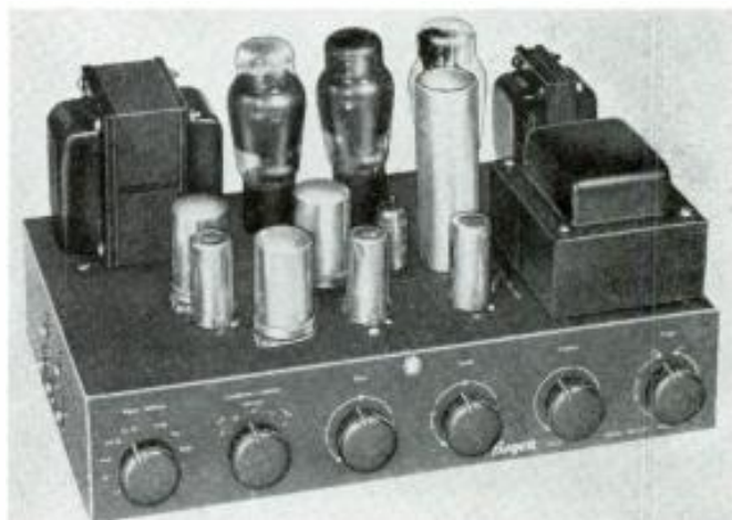
Amplifier-preamp combination features loudness contour selector.
