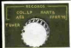
Control #1 Input selector Six positions: Tuner, Tape, AES, NARTB, FRFR, COL. LP. The latter four positions provide equalization for all records.
