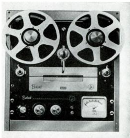
Berlant BR-1 professional recorder will hold five heads; takes NARTB reels; has easy loading, editing facilities; is portable.
