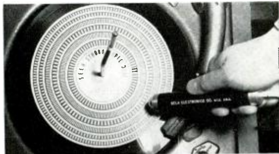
Special strobe flasher and disk make speed adjustment easy.
