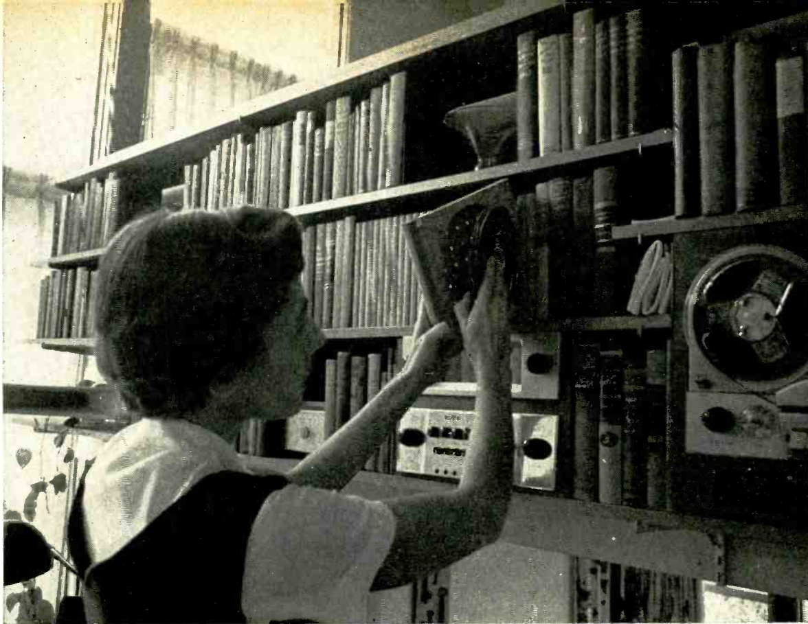
Eye-level mounting of equipment makes it easy to thread the tape recorder or lower the stylus on a disk.
