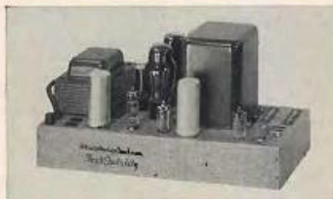
AP-428 POWER AMPLIFIER • Includes famous Stromberg-Carlson Duo-Power circuit. Peak power-handling capacity, 50 watts. Frequency response, 10 to 32,000 cps. Noise level better than 80 db. below rated output. Distortion, well under 1% at 25 watts. 4, 8, 16, 150 and 600 ohms and 8 VU output taps for tape recorder. 8 1/4" x 16" x 7". $95.00
