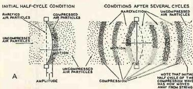
Fig. 2-1A, above: how a sound wave is produced. A vibrating string or diaphragm compresses the air particles in its path, and rarefies them in back. Fig. 2-1B, right: graphic picture of a sound wave.
