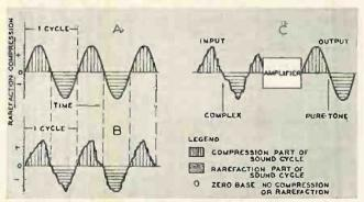
Fig. 2-3. A pure-tone (fundamental only) waveform is shown at A. At B is shown the same fundamental frequency with harmonics added, to make a complex tone. C depicts what happens to the complex waveform when it is passed through an amplifier that responds only to the fundamental frequency; such an amplifier would be said to have poor high-frequency response. Example is exaggerated, of course, for clarity.
