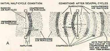
Fig. 2-1A, above: how a sound wave is produced. A vibrating string or diaphragm compresses the air particles in its path, and rarefies them in back. Fig. 2-1B, right: graphic picture of a sound wave.
