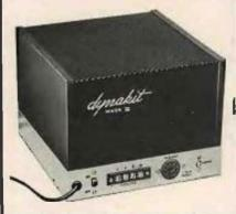
60 Watt Deluxe Model of the famous DYNA-KIT that has established new standards of clarity in reproduction. Instantaneous peak of 140 Watts—I M less than .05 at average listening levels—Choke filtering—hum and noise level 96 db below 60 Watts—new English KT-88 tubes for long, trouble free life—4, 8, 16 ohm taps. Bro- 579.95 chure available.
