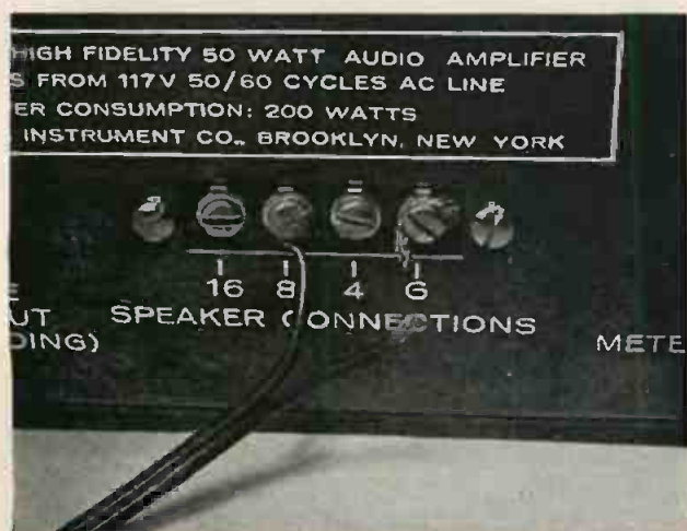
High-fidelity system failure may be due to nothing worse than a broken wire. Check all connections.
