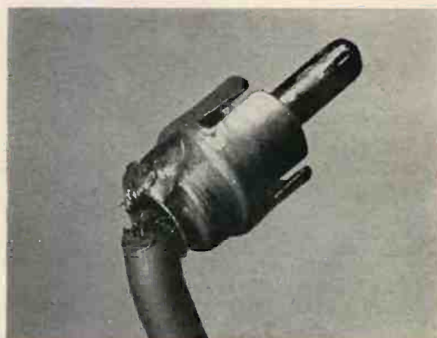
Hum can be caused by broken shield on connecting cable. A drop of solder will usually fix things.
