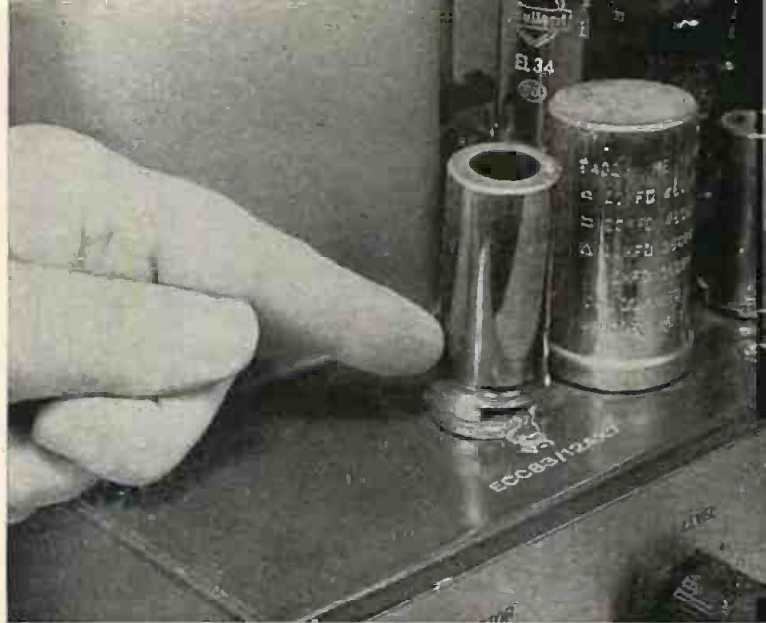
Tube shields which have become loose can cause hum and microphonics. Shield should be clamped tightly on base.
