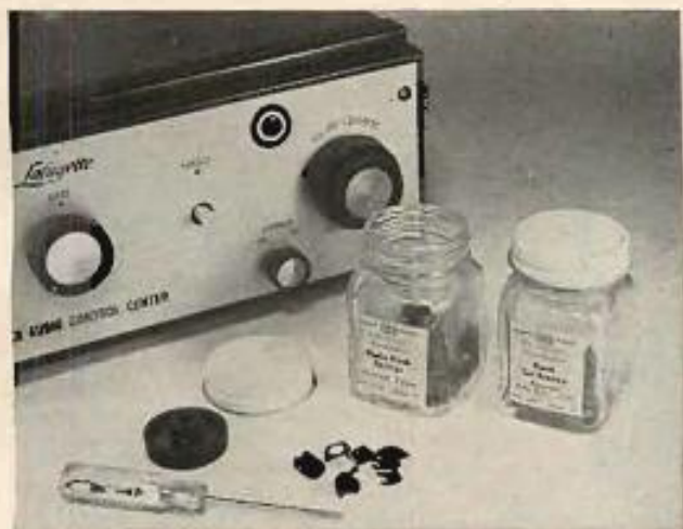
Control knobs are held in place by springs or small set screws, which come in assortments for quick replacement.
