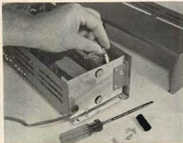
Replacing a pilot lamp is a simple task, once the bad bulb is exposed. Remove AC cord before dismantling.
