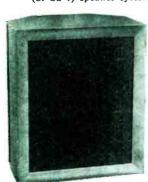
and a super tweeter to extend overall response from 35 to 16,000 CPS ± 5 db. Crossover circuit is built-in with balance control. Impedance is 16 ohms, power rating 35 watts. Constructed of 3/4" veneer-surfaced plywood suitable for light or dark finish. All parts precut and predrilled for easy assembly. Shpg. Wt. 80 lbs.
