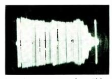
Sweep from 200 cps to 20 kc on Elektra 35 record. The GC-5 was connected to a preamplifier input for this oscillogram, which accounts for the evident peaking and rolloff at very high frequencies.
