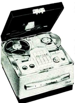
GUARANTEED SPECIFICATIONS—Playing time up to 4 hours, using LP tape 3½ ips, 7" reel. Frequency Response—Upper Channel: 40-15,000 cps. ±3db. at 7½ ips.; 40-8,000 cps. ±3db. at 3½ ips.; Lower Channel: 40-15,000 cps. ±3db. at 7½ ips. (NARTB Standard Equalization). Wow and flutter less than 0.3%; Signal to noise ratio greater than 50 db.; Signal from lower channel pre-amp output 0.5—1.5 volts; Crosstalk—50 db.
