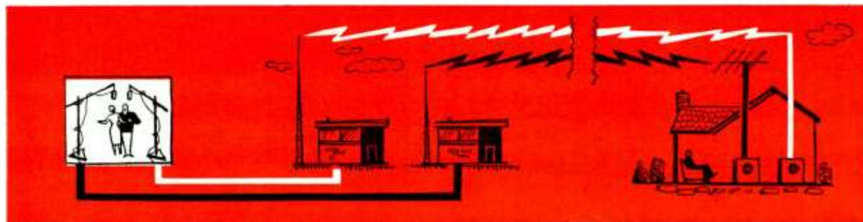
Stereo broadcasting starts with two microphones, goes through two complete sets of electronic facilities and out through two transmitters. Reception must be kept similarly separate: through two antennas and receivers into properly oriented loudspeakers.
