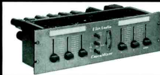
Model M-5: Five independent mixing positions plus master gain control. Phono equalizing and cueing switches on front panel for mixers 2 & 3. A 60db pad switch enables mixer-1 to accept a high level, low impedance source. Single channel output.
