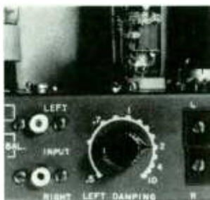
VARIABLE DAMPING To get the best from your speaker.
