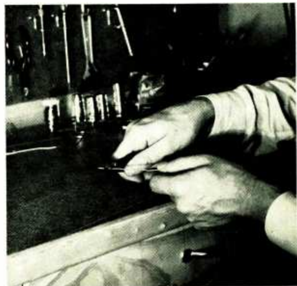
To "strip" a wire, remove a bit of its insulation.
