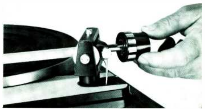
precision tonearm balance with rubber cushioned fine-thread rotating counterweight
