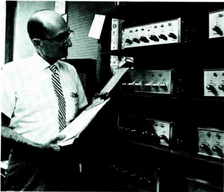
Victor Brociner shown at the "Life Test" Rack. Here production units are subjected to "on-off" cycles and voltages far in excess of those encountered in home use. Three months on this rack is equal to ten years of normal use.
