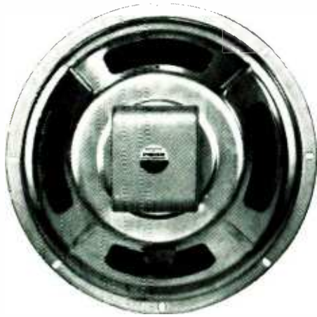
12" woofer with 6-lb. magnet structure, 2" voice coil, half-roll cotton surround, and 25 cps free-air resonance
