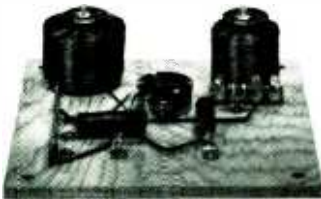
3-way inductive-capacitive dividing network with 1200 cps and 2800 cps crossovers, and continuously variable tweeter control
