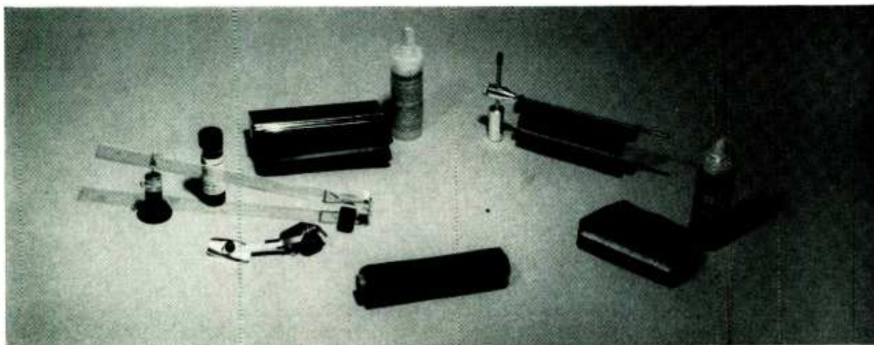
Newest devices include dust bugs in manual and changer versions, shown with Parastat above and Preener below. Upper right, Grado's Dustat; lower right, ADC Hush Brush.
