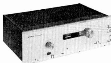
FM-3—STEREOMATIC FM tuner featuring automatic stereo/mono switching with the visual Stereocator. Super-sensitive, drift-free design with less than 0.5% distortion. Four IF-limiters, wide-band balanced bridge discriminator, and time switching multiplex.
