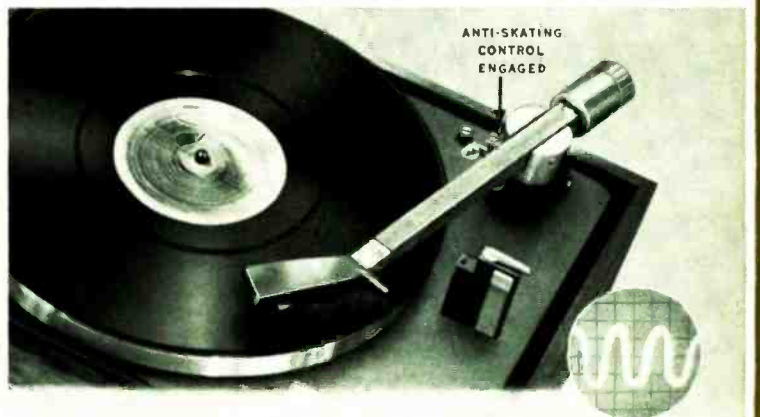
5 "Now watch me neutralize the skating force. I swing the anti-skating control back into position . . . and the arm tracks as perfectly as if there were a groove in the record! If I were playing a regular record—with the side pressure gone and resulting distortion eliminated—the sound would be cleaner."
