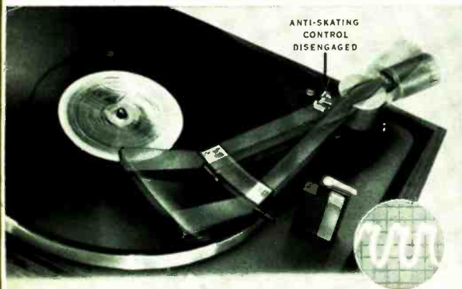
4 "Now you can actually watch the strength of the skating force. I start the Lab 80, but flip the anti-skating control over and out of operation. Note that as soon as I put the stylus on the grooveless record, the arm moves rapidly . . . with force, toward the center."
