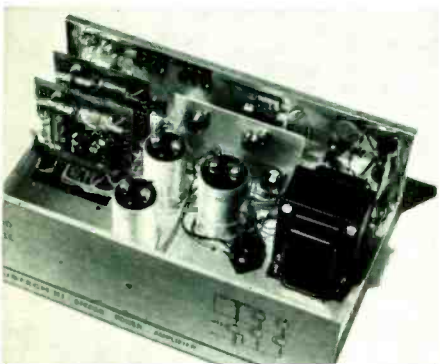
Step 1. Kit is designed so you can stop after wiring the easy-to-assemble power-amplifier stages, if you already own a hi-fi preamplifier. Construction time: about five hours.
