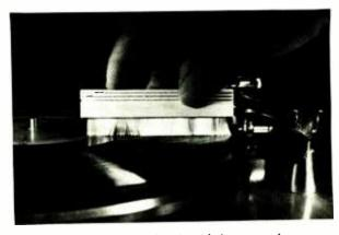
Holding the Parastat brush with just enough pressure to flex bristles helps clean record groove.
