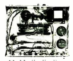
Open, uncluttered layout facilitates kit construction. Four etched circuit boards are factory assembled and tested.
