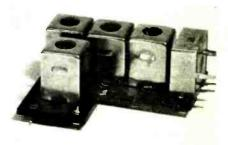
Improved Integrated Circuit AM: New Scott pre-tuned 4-pole LC filter improves AM selectivity; IC's and Field Effect Transistors in the AM section give better signal/noise ratio, lower distortion, and better signal handling capacity.
