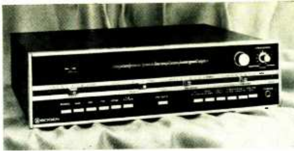
Crescendo control system on Bogen BR360 receiver, above, is designed to provide adjustment of dynamic range by offering volume expansion and compression. JVC/Nivico receiver, left, has built-in "Sound Effect Amplifier" that provides control over five frequency ranges, to compensate for room acoustics or speaker and pickup characteristics. Below, the Frazier Stereo Environmental Equalizer Model SEE-24, and a chart showing "before and after" response curves; the twelve adjustable circuit sections are intended to match a speaker's response to the room.
