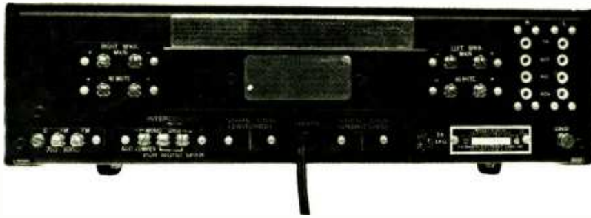
Uncluttered back panel of the Sherwood S-8900 has FM connections at lower left, preamp and control-section inputs at upper right, convenience outlets flanking line cord. Special feature is "mono spkr" (center-channel) output plus stereo pairs.
