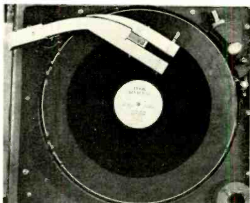
The Cook Laboratories binaural discs had to be played with this Livingston double-pickup arm. Signal for each ear was carried in separate groove, cutting playing time in half.
