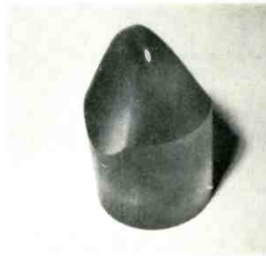
These models demonstrate the differences between the Shibata stylus (above) and the elliptical stylus (below). The sharply defined line toward the left side of the Shibata stylus is formed by the meeting of its two side planes and is on the trailing face of the stylus. The leading face is rounded.
