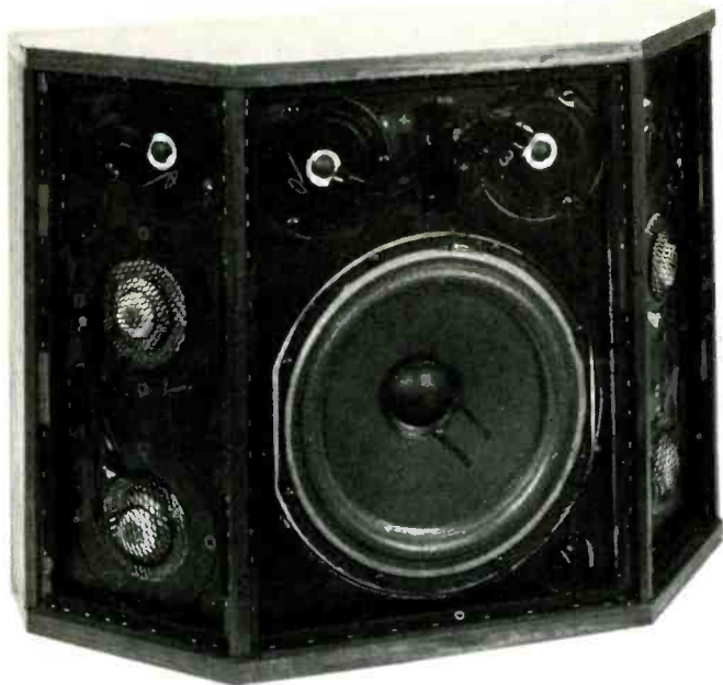
Tweeters of AR LST are the four drivers at the top of its three front panels. Woofer is in center panel; midrange drivers flank it in side panels.
