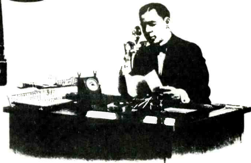
Poulsen's Telegraphone was conceived as an adjunct to the telephone—for dictation or for high-speed telecommunications. These illustrations from an early advertising piece show the special telephone equipment (resembling those in Poulsen's native Denmark) used in remote dictation.
