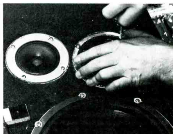
Today's typical kits—here represented by Heath AS-104—include a collection of parts (upper left) that must be assembled (upper right) to make crossover/control unit. Enclosure comes preassembled. Crossover unit is mounted at back, acoustic stuffing added (lower left), drivers mounted on front panel (lower left and previous page). When grille cloth is placed over drivers the system is complete.
