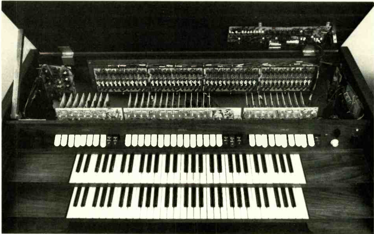
With hinged console lid raised, Recital's stop-filter boards are readily accessible. Library of Stops accessory kit permits wide variety of custom plug-in replacements to be constructed.
