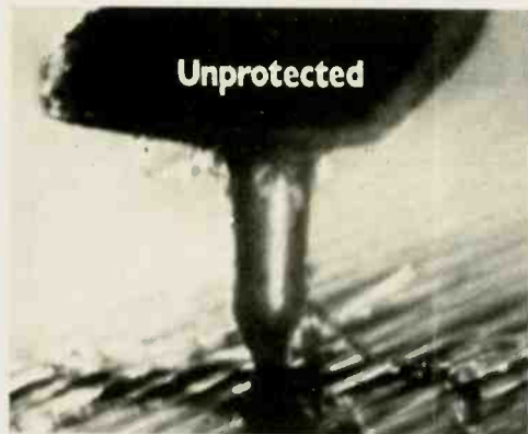
Magnification shows the record vinyl wearing away.
