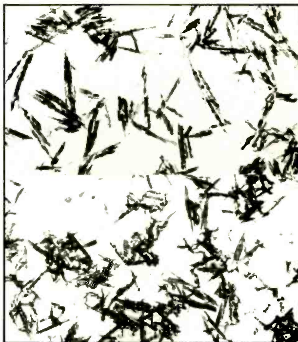
Photomicrographs from Ampex suggest differences between iron oxide (top) and pure iron particles. Ideal is small, well-proportioned "needle," consistent in size and shape, evenly dispersed, and randomly oriented in binder medium.
