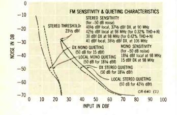
two. LOCAL, as the name implies, is for strong-signal reception. In normal operation, the tuner automatically chooses DX whenever the signal level is low.
