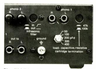
Others (this is Holman design for Apt) hide controls at the back as a set-and-forget onetime adjustment.
