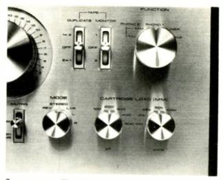
Some preamps (like this, in a Pioneer integrated amp) have phono-loading controls visible on the front panel.
