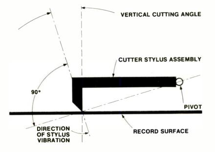
Fig. 2: Stylus assembly construction in cutting heads differs from that in playback cartridges, affecting to some extent the range of vertical cutting angles that can, in practice, be designed for. The cutting and playback angles should agree, however.
