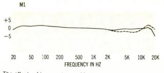
The effects of incorrect capacitive loading can be difficult to predict. With this particular pickup, the correct loading (450 picofarads) produces the fairly flat response curve represented by the solid line. When loading is reduced to 150 picofarads (dotted line), not only does a nasty peak appear at the top end, but the treble below the peak is noticeably weakened.
