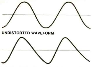
WAVEFORM WITH VTA-ERROR DISTORTION
