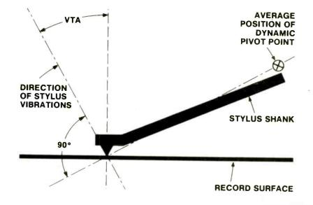
ate suggestion to the RIAA standards committee: Why not pick 15 degrees? This figure had the merit of being nearly midway between the extreme values of vertical angle, ranging from less than 0 degrees to more than 40, that were attributed to the various cutters and pickups then being used. And 15 degrees was not a difficult value to achieve in cartridge design—or so it was believed at that time.
