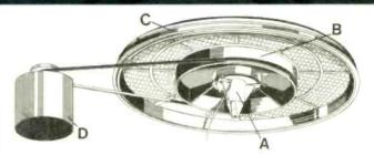
A 160 pole tacho generator (A) at the driving disc (B) electronically monitors the platter's (C) rate of rotation. The tachometer's d.c. signal is continuously compared to a stable d.c. reference signal. Any variations (+ or -) and the tachometer (A) instantly accelerates or slows the separate d.c. motor (D). Direct Control actually puts the driving disc into the electronic feedback loop for excellent speed stability.
