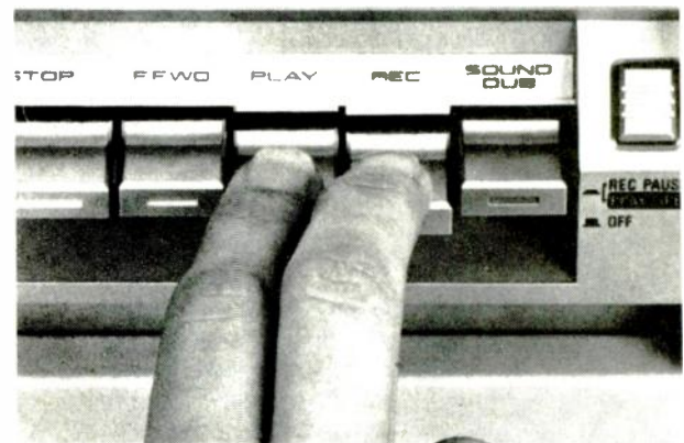
Controls are simple and straightforward. To record, you depress the PLAY and RECORD keys. Sound dubbing is also possible.
