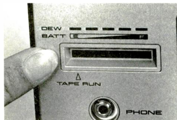
Thorough use is made of single LED panel, which indicates battery strength, proper tape run (LED at far left flickers), and moisture (dew) buildup on the head drum.
