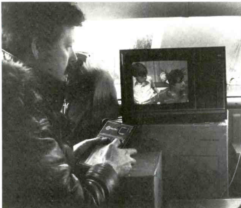
Backyard satellite antenna is oriented to one of a dozen satellites that maintain stationary positions thousands of miles above the Earth. Handheld switcher selects among satellites and allows viewer to pick any of twenty-four channels from each.
