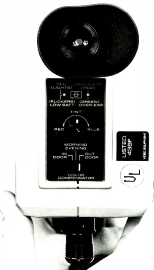
Control panel is on rear of camera. First set color compensator for lighting in use. Then turn tint control to fine-tune (see text).
