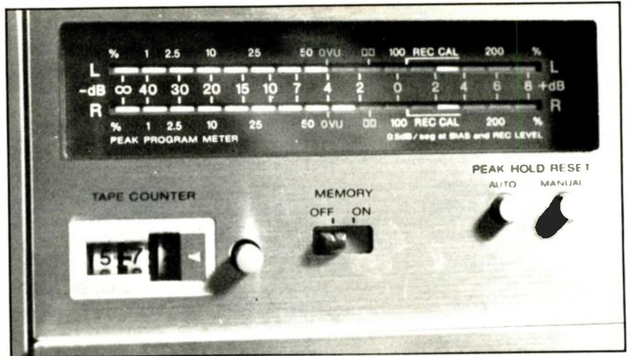
Level display's peak-hold cursors (here between +2 and +4 in both channels) retain maxima for a moment in AUTO mode to aid reading values. In MANUAL, readings remain until higher level occurs or display is reset, permitting unattended monitoring of maximum source levels.
