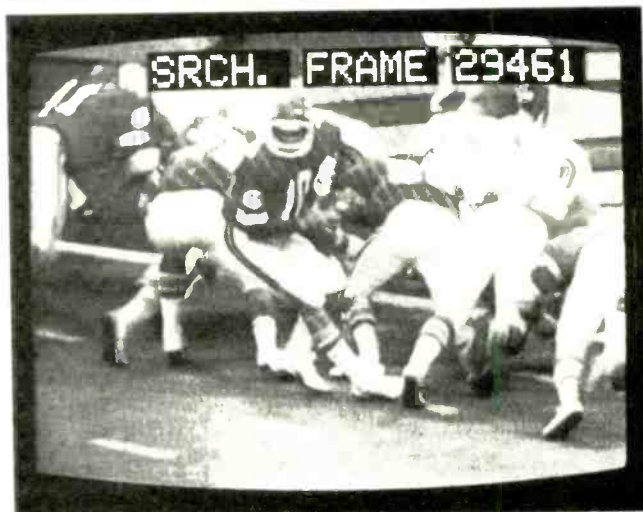
Among the many viewer-operated controls is SEARCH FRAME, which lets you locate a particular frame almost instantly. A total of 54,000 individual frames are contained on the disc.
