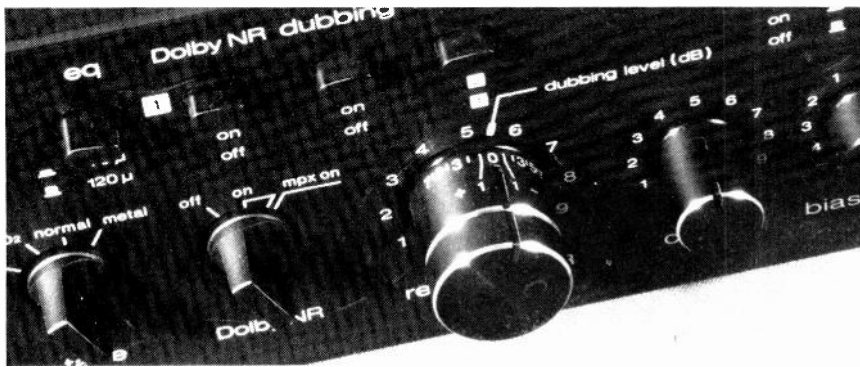
Recording level control calibration is unique. Copy levels will be identical to original (with appropriate tapes) when "0" on knob is aligned with dubbing mark on faceplate; other calibrations deliver measured changes in level where desirable.
