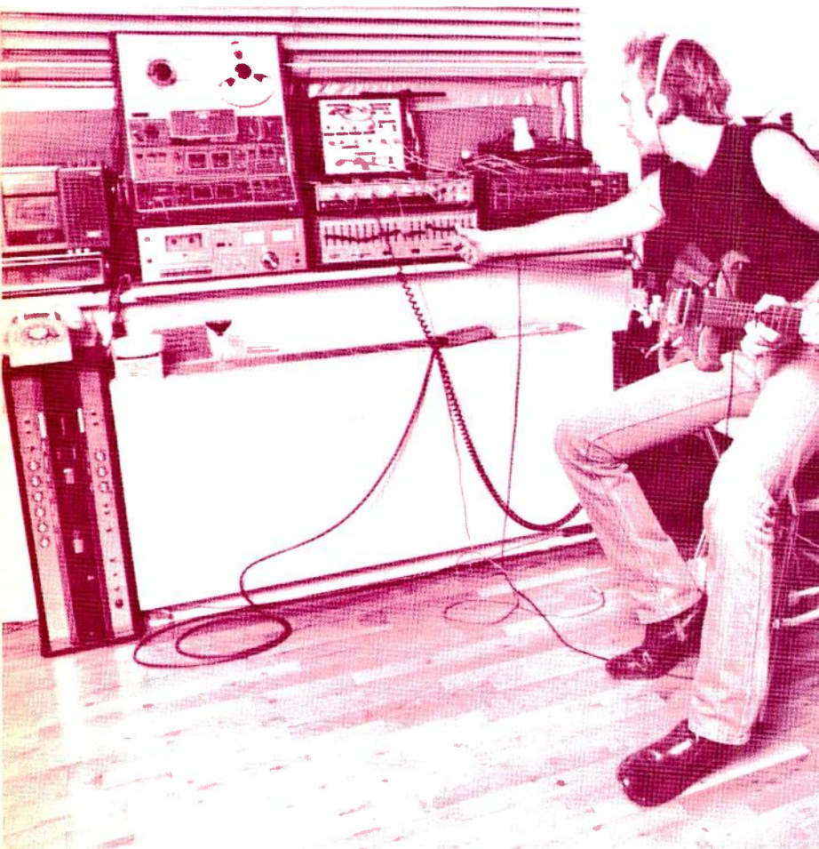
From left: Superscope portable, Sony TC-366 (top), Technics M-7 cassette deck, patch bay (top), Tapco mixer, Soundcraftsmen equalizer, Maestro phase shifter (top), Teac Model 1 mixer, the author at play
