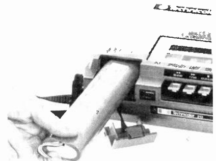
Flip up the cover and the rechargeable 12-volt nicad battery slips out easily. It's good for 40 minutes of power when used with the camera, so carry a spare.
