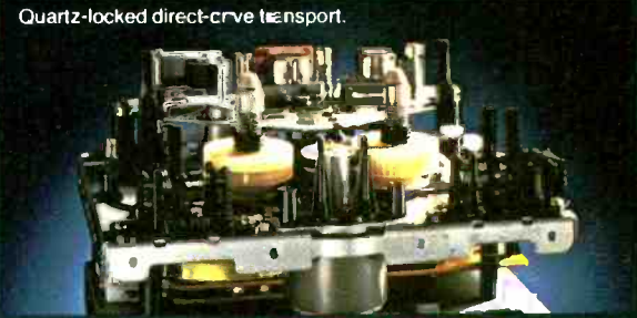
DD-7 with quartz-locked direct-drive.
