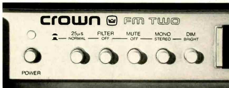
Crown FM Two's front-panel features include de-emphasis switch (for Dolby broadcasts) and dimmer for the front-panel display.
