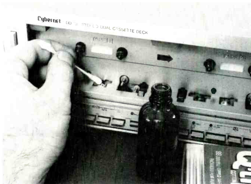
Cotton swabs and a bottle of pure isopropyl alcohol (not rubbing alcohol) can serve as a nearly universal head-cleaning kit for tape decks.
