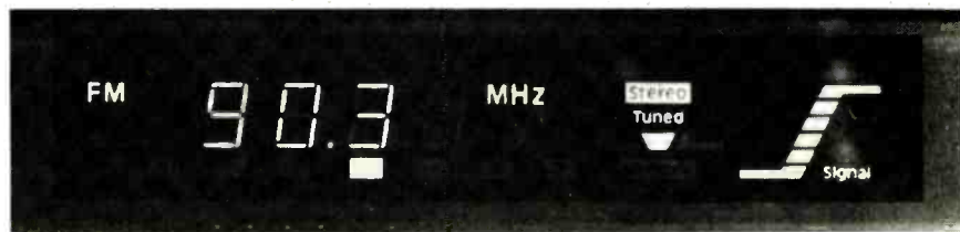
In the detail shown here, the 558T's neat visual display tells us at a glance that we're perfectly tuned to a very strong FM stereo broadcast on 90.3 MHz, which also happens to occupy the fourth memory preset position.
