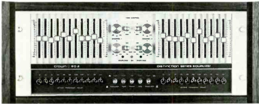
SAE's E-101 (top) is a two-band parametric with microprocessor controls; ten settings in each band can be stored in memory. Crown's EQ-2 is a ten-band parametric design, combining features of parametric and graphic equalizers.
