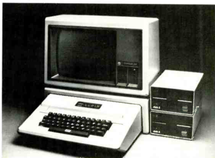
AN APPLE II PLUS computer readily performs music-filing chores. Two disk drives and a high-resolution monitor are necessary extras for this application.
