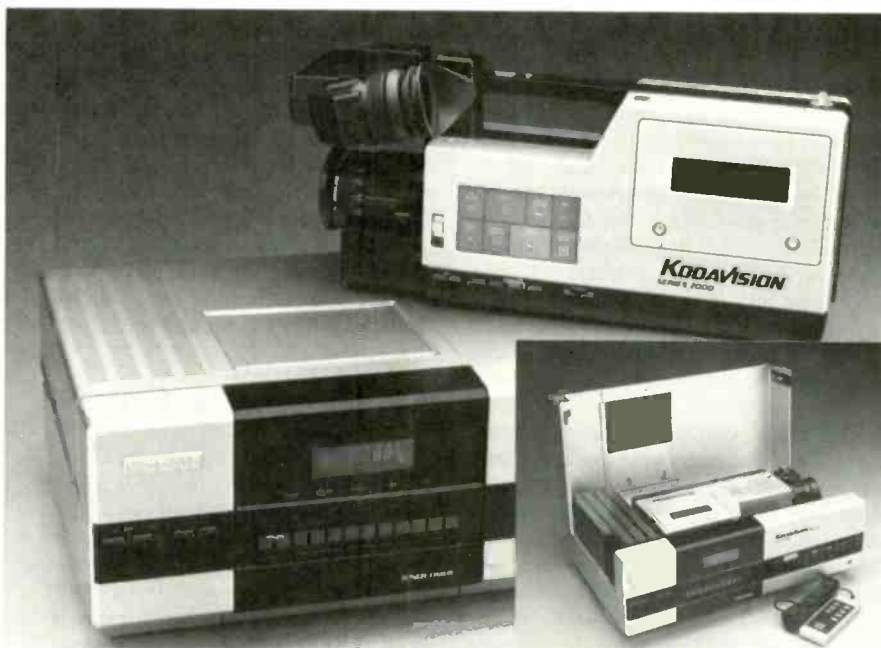
Kodavision 8mm portable video system: camcorder in cradle for home viewing (inset)
