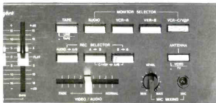
WITH THESE CONTROLS you can monitor the output of three video sources, dub between two VCRs, make two simultaneous copies of a third source, select between two audio soundtracks, perform audio-video fades, and add voiceover.
