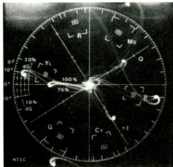
COLOR ACCURACY of the AVS-2100 is very good. The vectorscope photo at left indicates excessive color saturation (chroma level) and a very small amount of hue (chroma phase) error. The photo at right—made with a 3-dB cut in chroma level and a clockwise phase rotation of approximately 4 degrees—simulates the best results obtainable using the color and tint controls on a monitor. This puts all six color vectors (white dots) on their targets, which is near-perfect performance.
