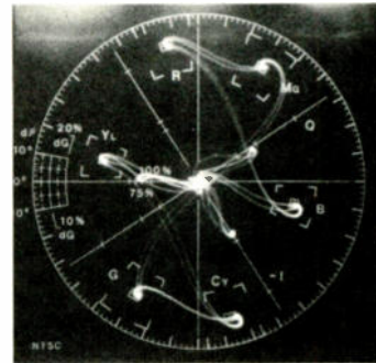
COLOR ACCURACY of the AVS-2100 is very good. The vectorscope photo at left indicates excessive color saturation (chroma level) and a very small amount of hue (chroma phase) error. The photo at right—made with a 3-dB cut in chroma level and a clockwise phase rotation of approximately 4 degrees—simulates the best results obtainable using the color and tint controls on a monitor. This puts all six color vectors (white dots) on their targets, which is near-perfect performance.
