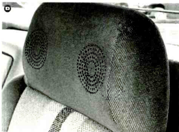
A PONTIAC FIERO gives you enough vertical dash space to mount an equalizer atop the front end (A, B). Dash-mounted speakers provide volume and bass (C), while the FIERO's optional headrest speakers give a nice spatial quality (D).
