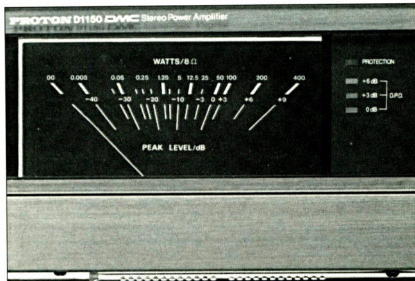
The AA-1150's level meters are supplemented by three peak-indicating LEDs (right).
