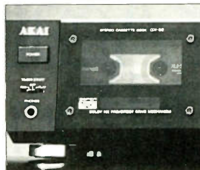
The GX-52's motorized cassette-well door
