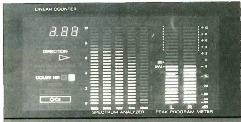
The TC-RX80ES's display contains a five-band spectrum analyzer (center).
